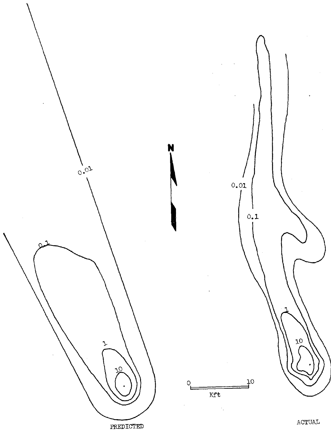
Figure 44. CABRIOLET fallout pattern as predicted by NCG scaling model. Exposure rates at H+1 in R/hr.
